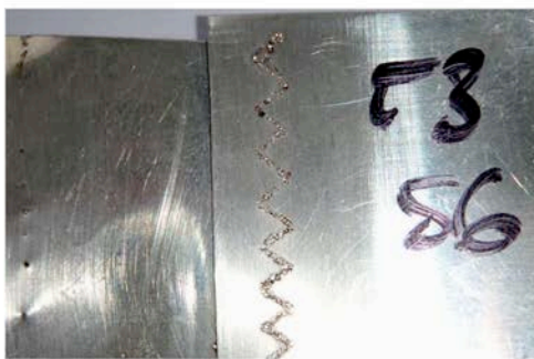
Example 2b: Welding two sheets flat (zigzag)
