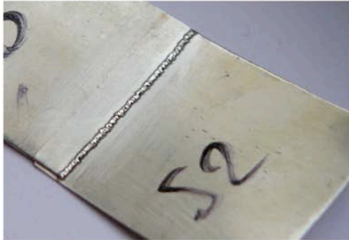
Example 1: welding two sheets over edge
